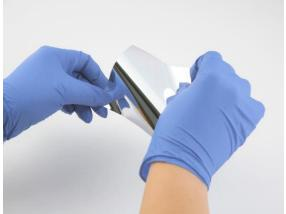
Deposition Sciences, Inc., a wholly owned subsidiary of Lockheed Martin, specializes in advanced materials and optical coatings. For over 20 years, they've been producing their Sunshade® thermal control material, which is designed to provide reliable performance in extreme space environments.
