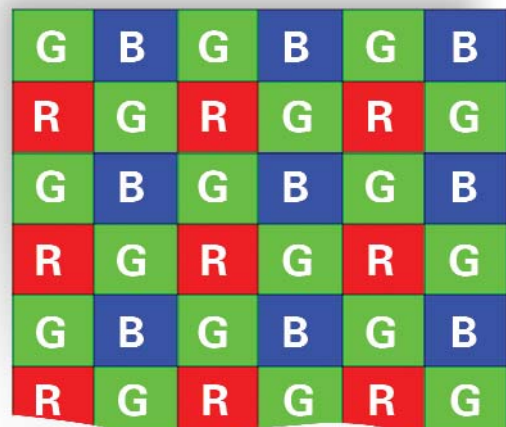
FIGURE 1. THE RED, GREEN, AND BLUE INFORMATION IS INTERPOLATED ACROSS SEVERAL ADJACENT CELLS TO DETERMINE THE TOTAL COLOR CONTENT OF EACH INDIVIDUAL CELL.
