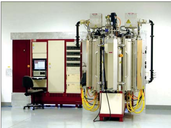
FIGURE 6: THE MODEL 67242 MICRODYN® SPUTTERING MACHINE IS A FULLY AUTOMATED MACHINE WITH TWO DOORS, FOUR 40-INCH CATHODES, TWO MICROWAVE PLASMA SOURCES, AND A BLANKED-OFF PORT THAT IS AVAILABLE FOR MOUNTING A FIFTH CATHODE, HEATERS, DIAGNOSTICS, ETC.
